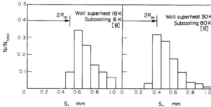
FIG. 1. Distributions of nearest-neighbour distances, flow boiling of water on stainless steel.
