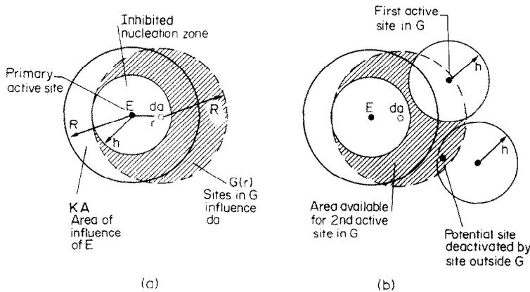
FIG. 4. Model for calculation of overlap with inhibited nucleation zone.
