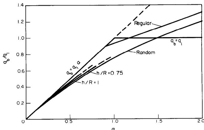
FIG. 3. Effect of overlap on boiling heat flux.
