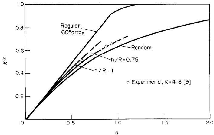
FIG. 2. Effect of overlap on true boiling area.
